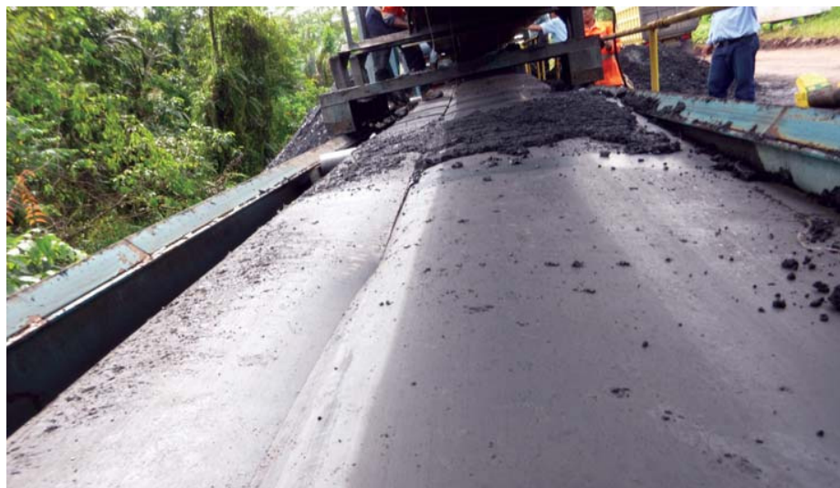
Flexco was able to repair a conveyor tear (above) at Adimitra Baratama Coal's operations using Flexco Bolt Solid Plate 190 fasteners (below).
