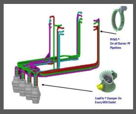
The closed-loop control system represents a world first for fuel balancing. Under different loads, coal-fired electricity generating units face an imbalance of the air-to-fuel mixture at the burners located on the boiler. The auto control units address this imbalance of fuel at each and every load, continually monitoring the system and making fine adjustments when needed to optimise fuel flow to the burner.
